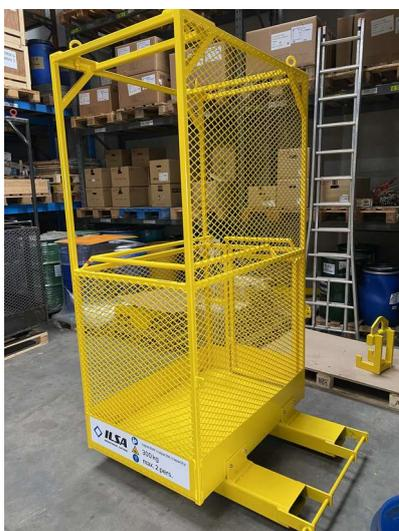
Man basket for use with forklift truck and for lifting
